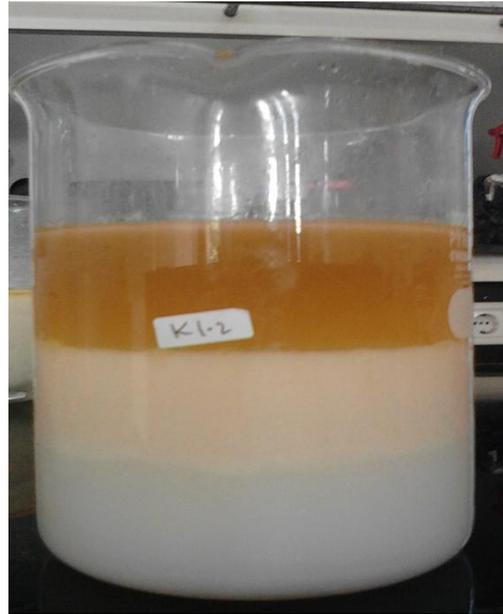
Gambar 5: pencucian biodiesel jelantah
