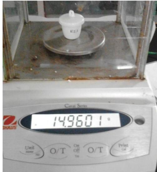
Gambar 10: pengujian kadar air biodiesel jelantah
