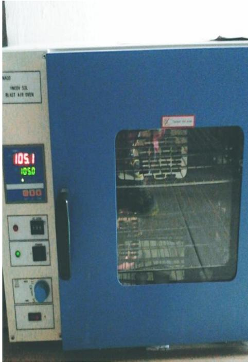
Gambar 11: pengopenan biodiesel
