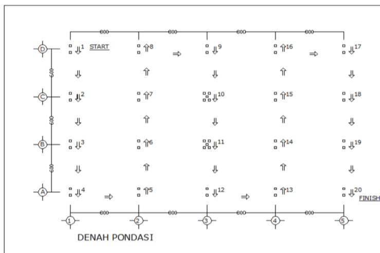
Gambar 10.3: Arah kerja mesin pancang drophammer
