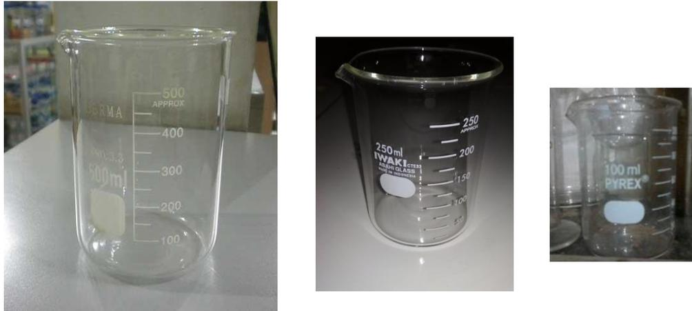
Gambar 3. Bekerglass 500 ml, 250 ml dan 100 ml (Sumber: Laboratorium Kimia
